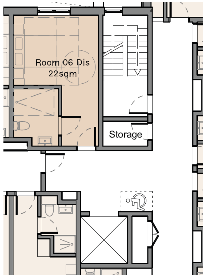
Figure 14: Accessible Rooms and Circulation Layout
