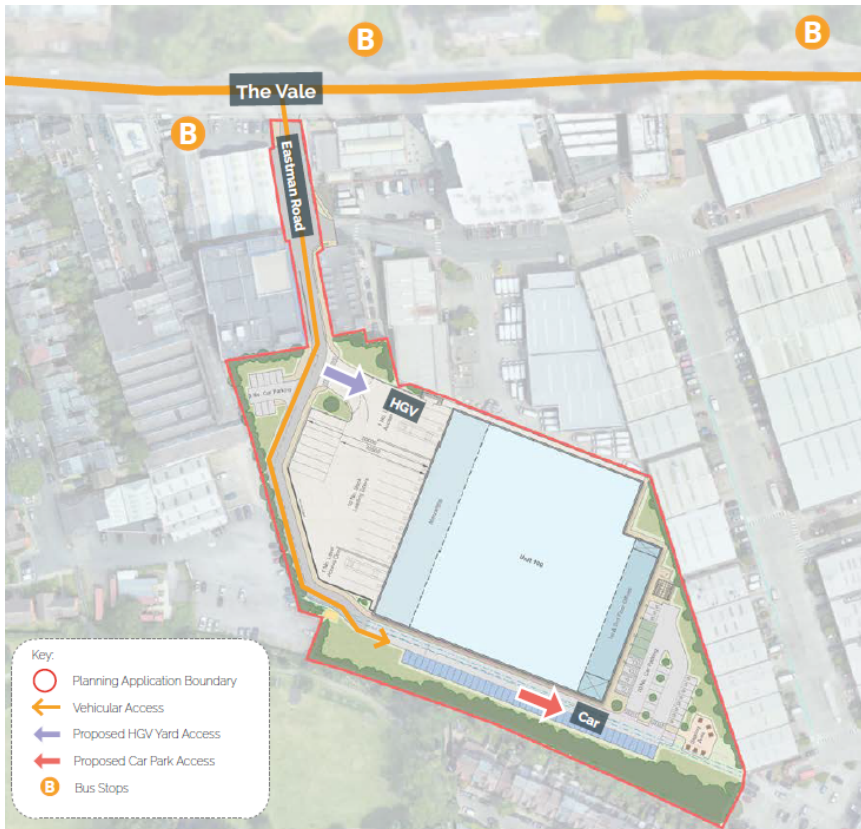
Figure 9: Vehicular Access Plan
